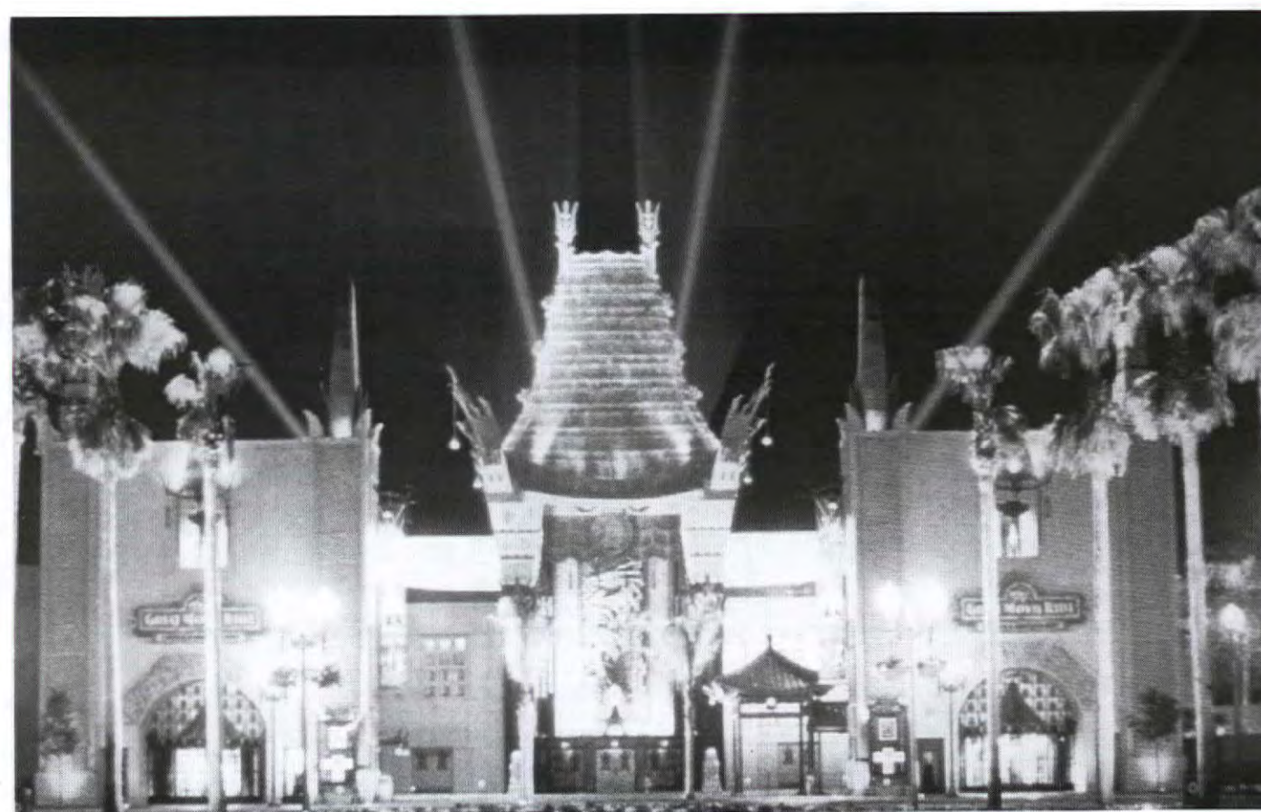
. . . Disney's version on "Hollywood Boulevard" at the Disney-MGM Studios Theme Park in Orlando, Florida, based on measured drawings of the original but not a museum-caliber replication. GFRP has replaced cement plaster walls; plaster painted verdigris has replaced the copper roof.
