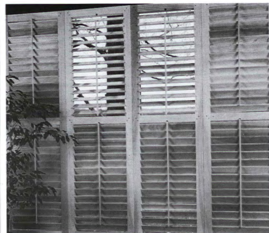
KESTREL MANUFACTURING produced these hardwood, bi-fold movable-louver interior shutters, using blind pocket, mortise-and-tenon construction, with tenons secured in the mortise with through-pegs. Louvers are attached to the louver tilt rod with solid brass threaded eyelets. Write in No. 799
