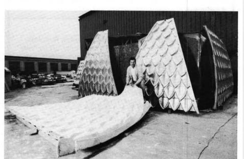
Replacement of exterior dome panels for the Garfield Park Sports Complex, Chicago, used mold rubber from SMOOTH-ON, INC. Shown are replacement panels, cast in GFRC. Write in No. 65
