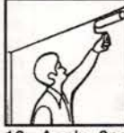
12. Apply 2nd coat of saturant (include seam)
