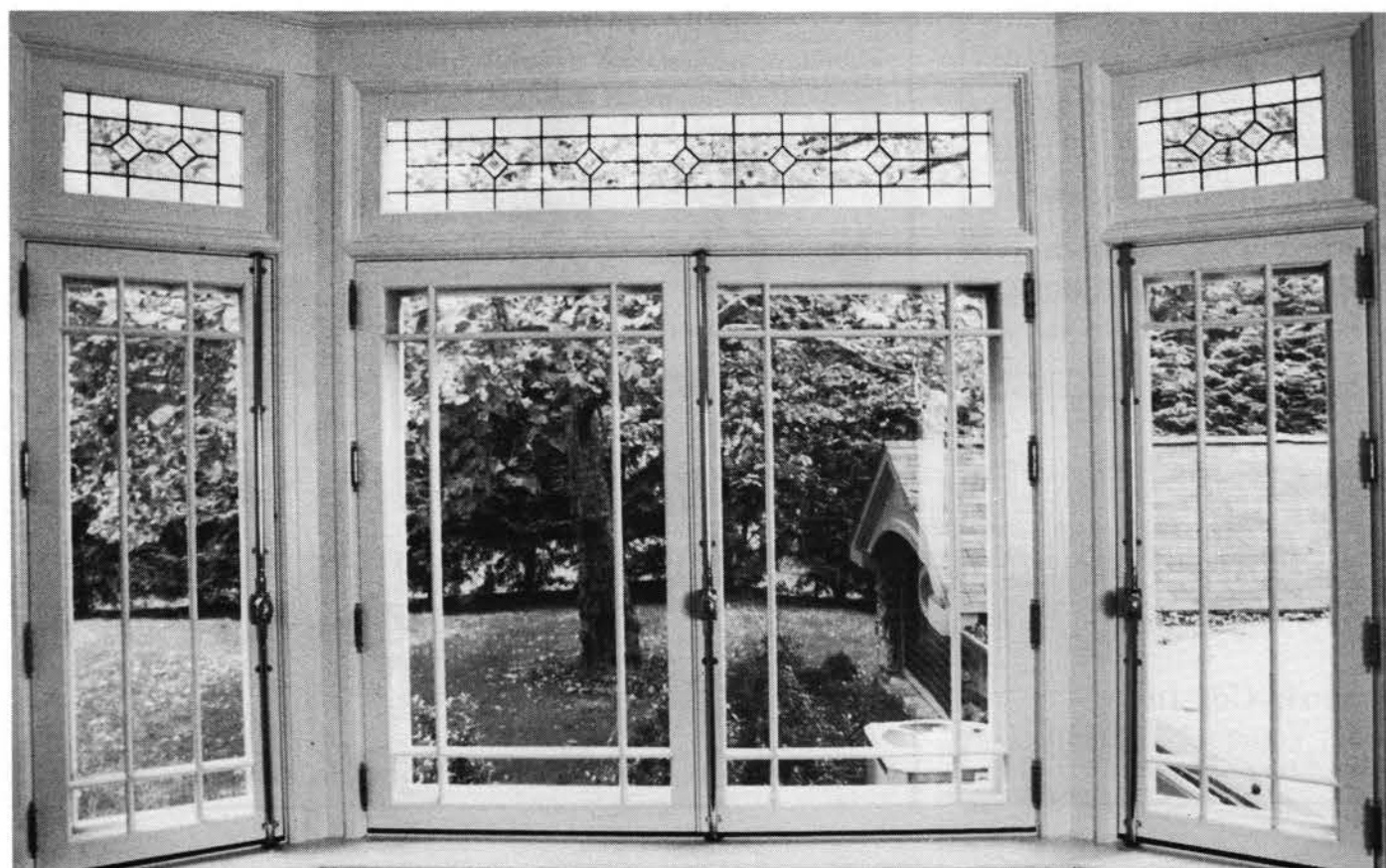
WOOD WINDOW WORKSHOP produced these custom mahogany French casements with true divided lites and single pane restoration glass. They feature 7/8 in. muntins, solid-brass hardware, and bronze interlocking weatherstripping. Write in No. 964
