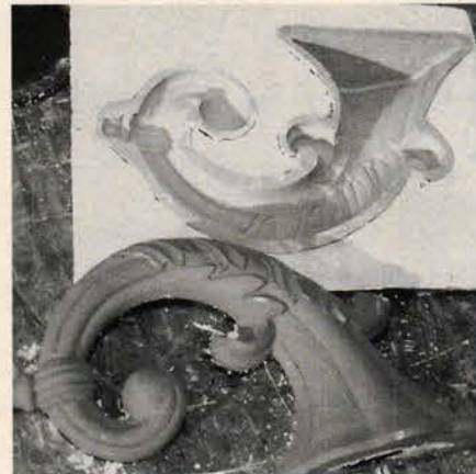
New York's Russian Tea Room turned to DUOMATRIX for the restoration of architectural ornaments: Matrix-G, mixed with Brass Powder, was brushed into a Smooth-On urethane mold; backed up with straight Matrix-G and glass fiber, it yielded the element shown here. Write in No. 811
