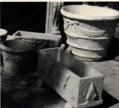
Concrete decorative items made for homes, upscale department stores, hotels, etc. duoMatrix-C added to the concrete mix reduces cure time, thereby increasing production rates. Elements are stronger (breakage in transit greatly reduced) and last longer due to reduction in water/salt absorption.
