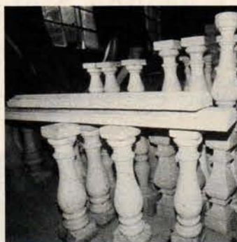
Concrete decorative items made for homes, upscale department stores, hotels, etc. duoMatrix-C added to the concrete mix reduces cure time, thereby increasing production rates. Elements are stronger (breakage in transit greatly reduced) and last longer due to reduction in water/salt absorption.
