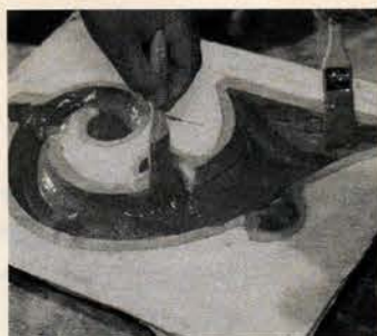
Architectural elements being made for the restoration of Manhattan's Russian Tea Room. duoMatrix-G system is mixed with Brass Powder and brushed into a PMC-724 rubber mold. It is then backed up with straight duoMatrix -G and glass fiber, yielding a strong, lightweight decorative item ready to be polished and mounted.
