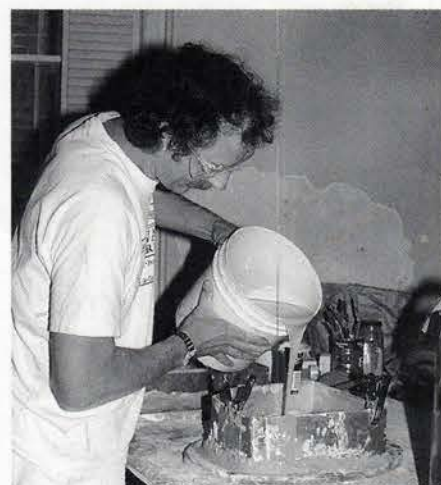
RORY BRENNAN pours rubber for a mold with which he will replicate a plaster original. Write in No. 2980
