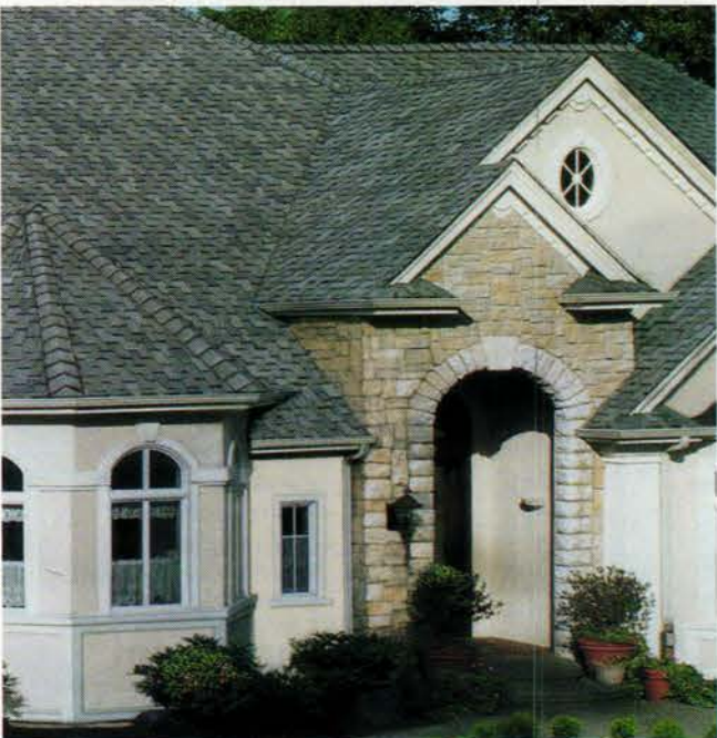
Grand Sequoia shingles from GAF MATERIALS CORPORATION reproduce the profile and texture of wood shakes, but have a UL Class A fire rating. The shingle's shadow effect and double-thick tabs create depth, and carved edges provide the random appearance indicative of wood. The shingles have a 40-year limited transferable warranty.
