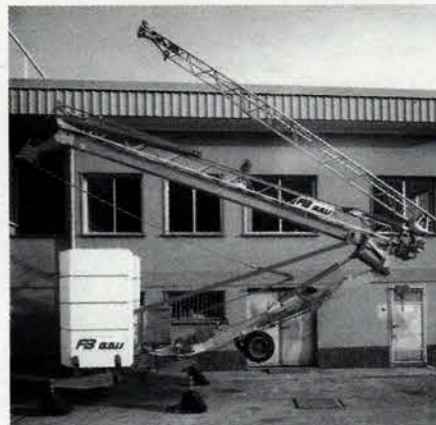
TOWER CRANES' compact "GA" cranes automatically position and level themselves thanks to the hydraulic equipment in their towers. Write in No. 77
