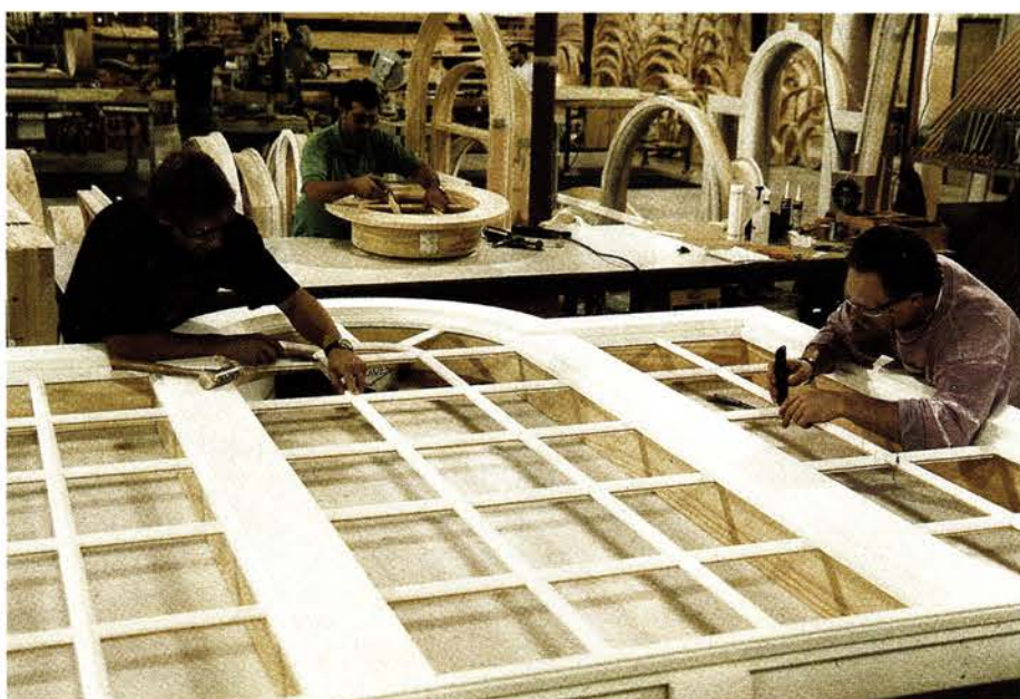
PARRETT MFG. fabricates custom windows in non-standard sizes and shapes, such as this divided-lite Palladian model. Write in No. 5005
