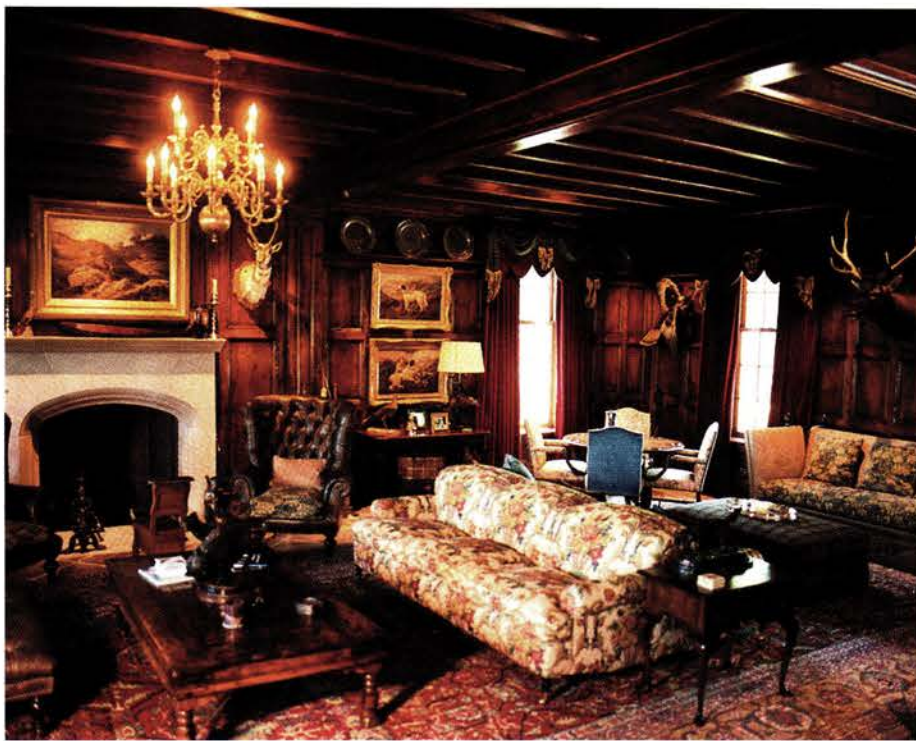
LANDMARK FINISHES created an English manor-style appearance for this room by distressing the knotty pine and then using multiple coats of shellac and a hand-rubbed wax. Write in No. 1686
