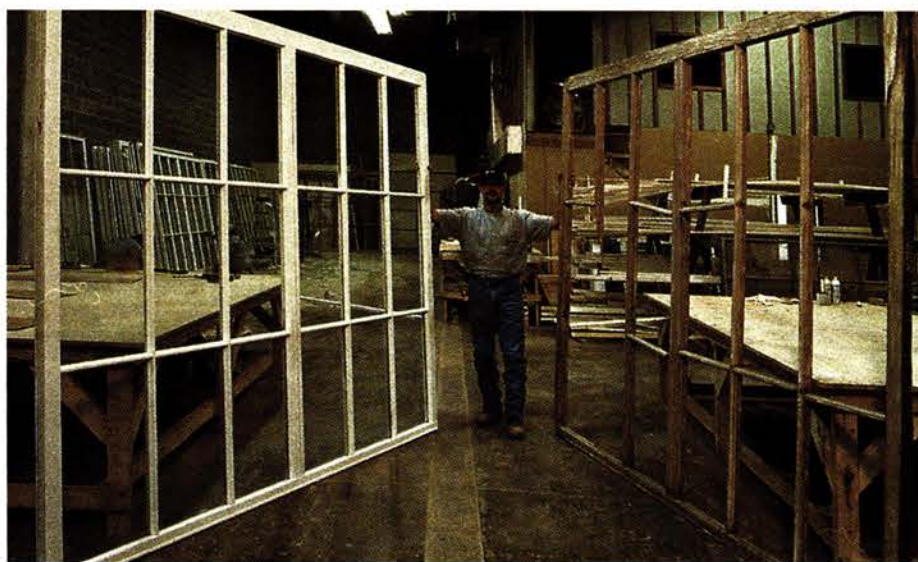
RE-VIEW restored 144 8x8-ft. triple-hung sashes for the Renaissance Grand Hotel in St. Louis, MO. Write in No. 744
