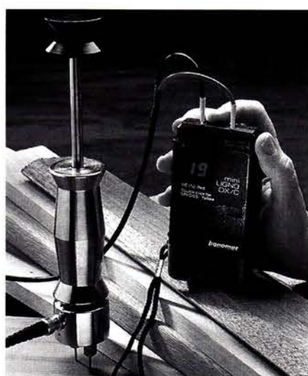
The mini Ligno DX/C from LIGNOMAT USA is used to detect moisture in wood and other soft building materials. Write in No. 1120
