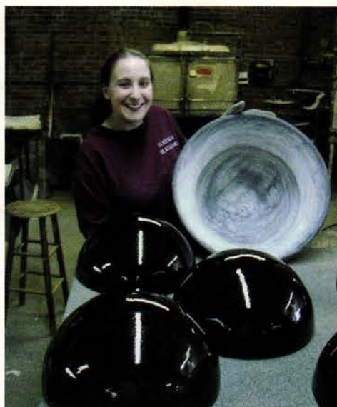
Thousands of steel molds, both antique and new, are kept on hand at Flickinger Glassworks. Rose Battah, one of the firm's expert glass benders, is shown here holding the mold used to cast the deep-amber bowls before her. These glass half-spheres were subsequently installed on the ceiling fixtures of the Legislative Services Building in the New Jersey State House.
