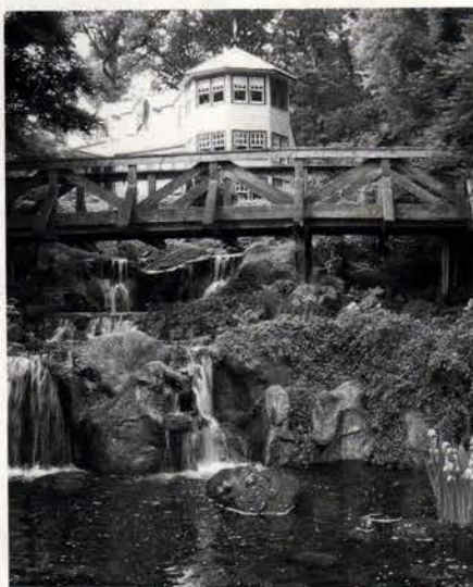
Waterfall Creations used natural and simulated rock, mixed on site to match the color of the natural rock, to create this series of waterfalls, streams and ponds.
