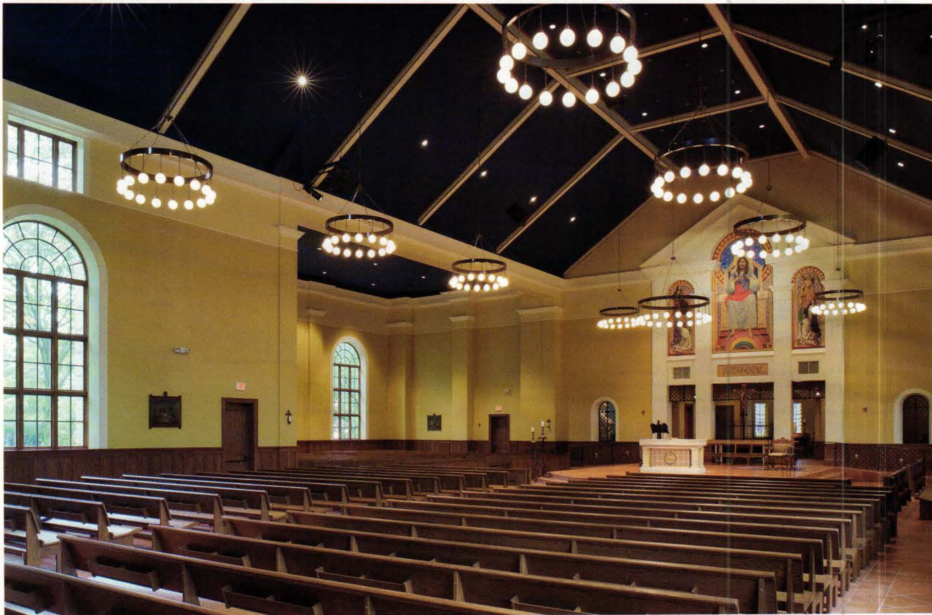
In the nave of the church (above and left), which seats 900, cost-saving measures included the introduction of a partially flat ceiling in lieu of a full cathedral ceiling to allow mechanical systems to be housed in the concealed truss space. The acrylic murals behind the altar were painted by Columbus-based artist Michael McEwan.
