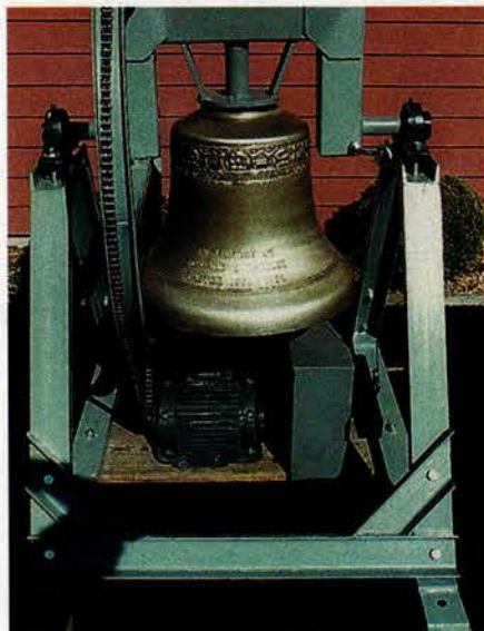
Elderhorst Bells outfits new and used bronze bells with either traditional rope swings or electronic swinging systems.
