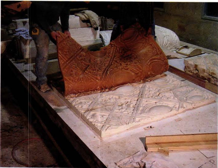
Rubber molds for the GFRF were cast from the assembled plaster masters.
