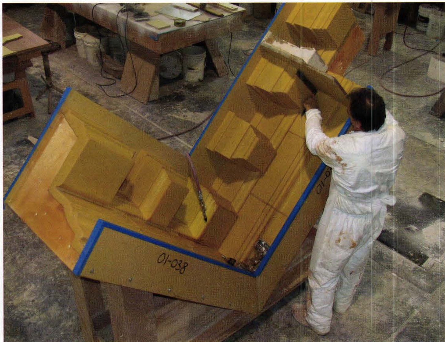
This rubber mold is being set up by Architectural Reproductions in order to produce a corner segment of a cornice. A modular approach is being used, with the multiple blocks ganged together in a modular mold with molded-in false joints. Photo: courtesy of Architectural Reproductions
