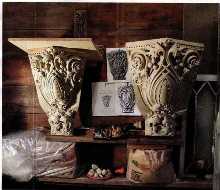
Among the few legible period images of the cornice was a close-up of a capital section, published in Architectural Record . Artisans transformed the grainy photo into deeply incised clay masters.
