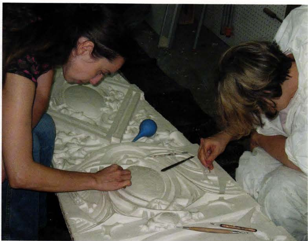
As masters for the GFRF were prepared, plaster models for the rubber molds were meticulously sanded and scraped.
