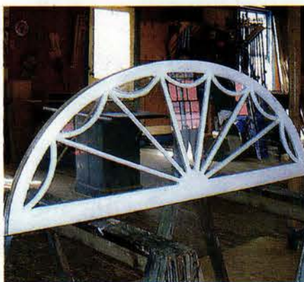
Jim Illingworth Millwork manufactured this attic half-round window sash with spiraled web using single-pane glass and true divided lites.
