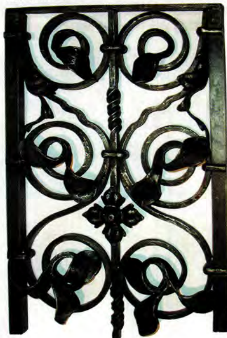
This forged scrollwork panel is one of 26 that were fabricated by Fine Architectural Metalsmiths as part of a monumental gate; it is made of pure iron and features repousse rosettes.
