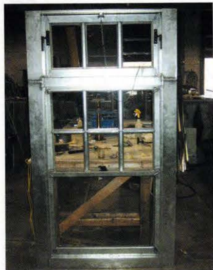
This hollow metal window was built by Heather & Little for the Robeling Museum in New Jersey.
