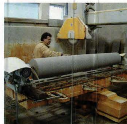
A column shaft of Indiana limestone is being turned on a lathe operated by a craftsman in the 20,000-sq-ft. studios of Traditional Cut Stone, Ltd.
