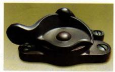
The model #LKF18 sash lock from Phelps Company is hot forged from solid brass and hand finished; the internal double-spring mechanism is made of stainless steel.
