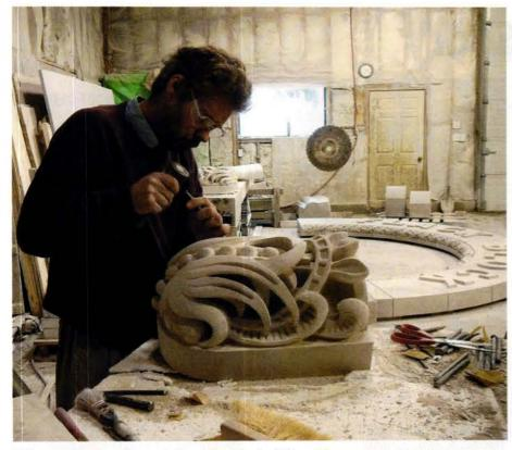
Artisans in the Canadian workshop of Architectural Stone Masonry work on aspects of the recreated entry for Vancouver's Flack Block. "It was all done by hand," ASM founder Tony Rogac says. "No machine touched any of that stone." The detail shows the careful hammer-and-chisel technique needed to produce an intricate, finely detailed ornamental piece.
