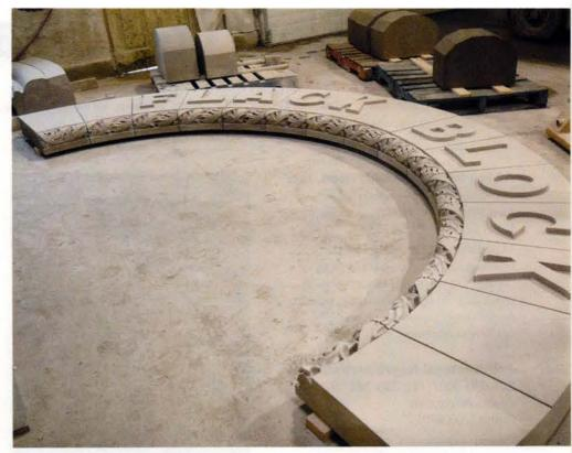
The original 20-ft. arch for the Flack Block bearing the building's name was re-created in the workshop of Architectural Stone Masonry. The new arch, like all the rebuilt elements, was sculpted in Indiana grey limestone because the original sandstone quarry that had supplied the first arch and its carvings was exhausted years before. Divided into 15 sections and adorned with a lower ornamental arc, the arch will again become a defining feature of its Vancouver streetscape once it's set in place.
