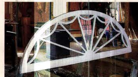
Illingworth Millwork manufactured this attic half-round window sash with spiraled web using single-pane glass and true-divided lites.
