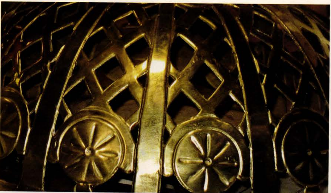
To replicate the remaining “crown and basket” fixture, Aurora used an old-world chasing and repousse process: a clay-like substance called “pitch” was used to make a mold, then artisans created the delicate piercings and embossed patterns by hand. Photos: Aurora Lampworks
