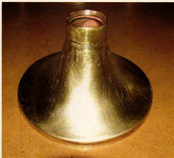
Aurora carefully removed the corrosion, matched missing metal pieces, then brushed and refinished each fixture. Photos: Aurora Lampworks
