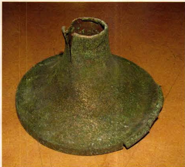
Aurora carefully removed the corrosion, matched missing metal pieces, then brushed and refinished each fixture. Photos: Aurora Lampworks
