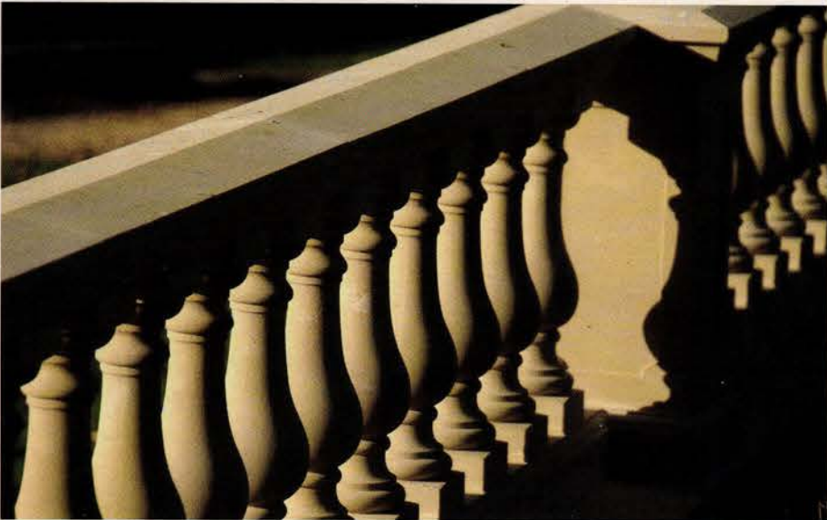
Haddonstone (USA) 's cast-stone balustrading can be formed into straight, ramped, curved and spiral configurations and used on steps, balconies and parapets. Key in no. 4020
