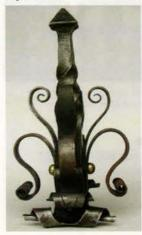
This crown finial was forged by the artisans at Fine Architectural Metalsmiths as part of the reproduction of an historic gate; it is 14 in. tall and features four-sided forged scrolls wrapping a center finial on an incised, rolled sheet-iron base.
