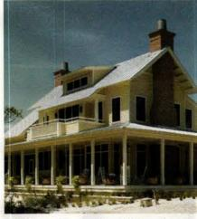
FiberCement siding from CertainTeed is made of recycled fly ash, Portland cement, wood fiber and additives.
