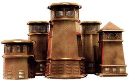
Jack Arnold-European Copper offers five styles of copper chimney pots measuring up to 3½ ft. tall; they are designed to prevent rain damage and animal infestation while improving draft and reducing the risk of fires.
