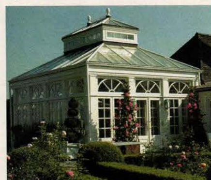
British bespoke hardwood conservatories from Oak Leaf Conservatories are constructed of mahogany with high-performance double glazing.
