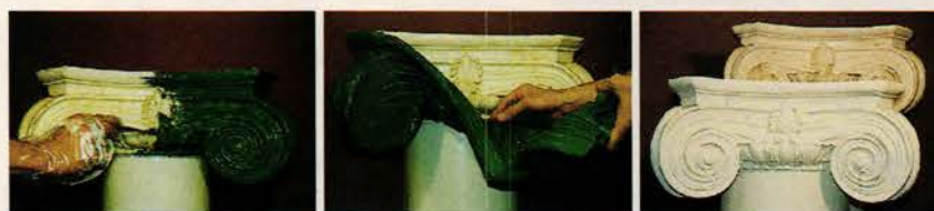
MasterMold can reproduce capitals, structural and decorative components, statuary and other patterns precisely and cost-effectively.
