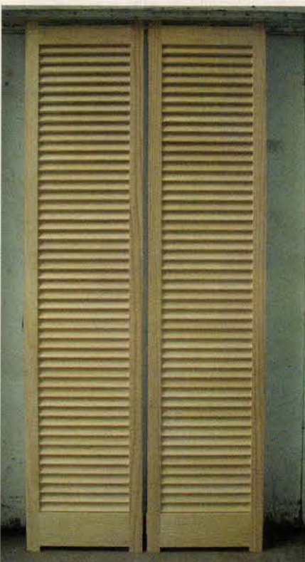
Weston Millwork built these replication stationary-slat blinds using mortise-and-tenon construction and matched the original thickness, width, spacing and angle of slats.
