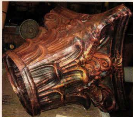
Heather & Little made these 24-oz. copper capitals for the restoration of Milwaukee City Hall.
