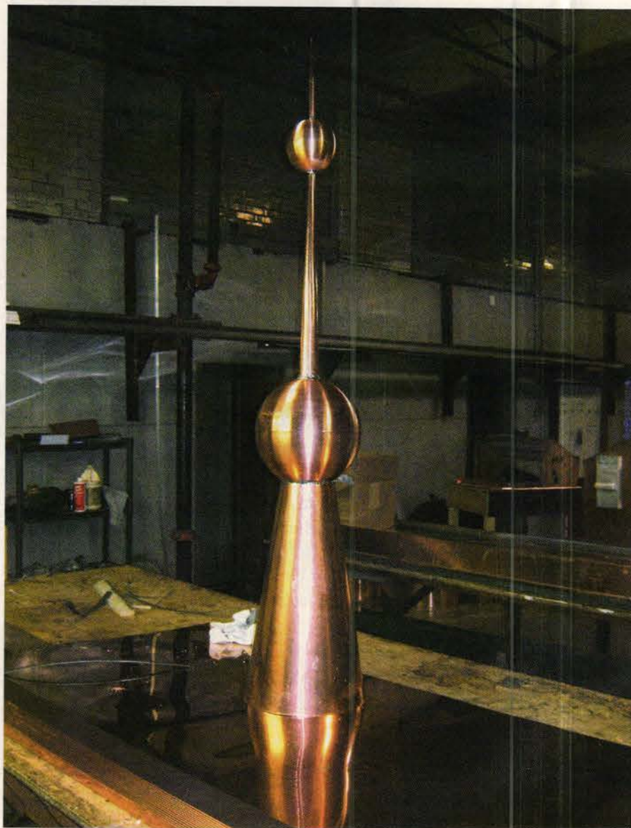
A 5-ft.-tall finial was hand-soldered together using copper balls, supplied by Nevada, MO-based W.F. Norman, and cones.
