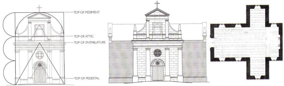
Through meticulous research, the architects found that historically, the main facades were much more dramatic when compared to other parts of the structure. Therefore, the main façade was veneered in stone-like lime stucco with Tuscan columns while the rest of the exterior and interior are relatively modest designs. Rendering and drawing: courtesy of Mesick, Cohen, Wilson and Baker Architects
