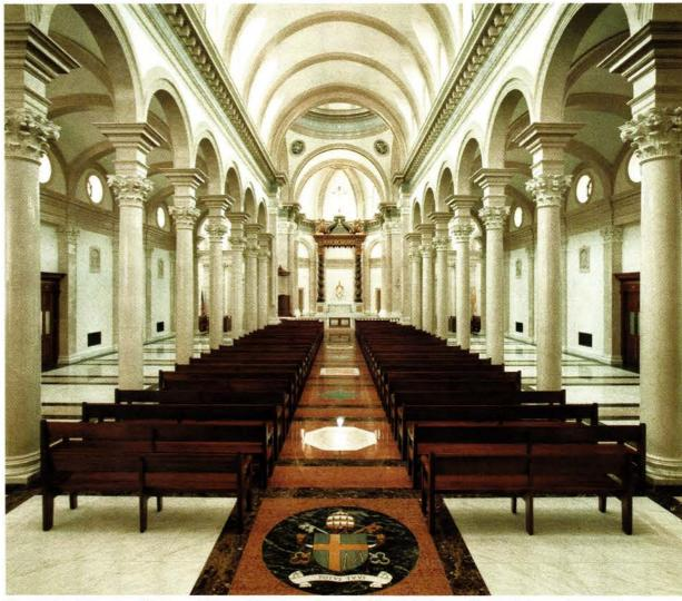
The interior of the chapel features 16-ft. marble columns (including the Botticino marble shaft, Apuano base and plaster capital) on either side of the nave, wide side aisles, a vaulted ribbed ceiling and an inlaid marble floor that leads the eye to the altar and tabernacle. Lighting is primarily from the clerestory windows, with recessed uplights in the cornice. Photo: Stephen Schafer, Schaf Photo Studios
