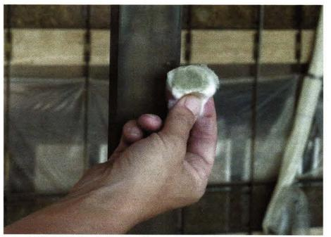
A cleaning test at the theater illustrates the corrosion and soiling that have accumulated over the original oxidized metal finish.
