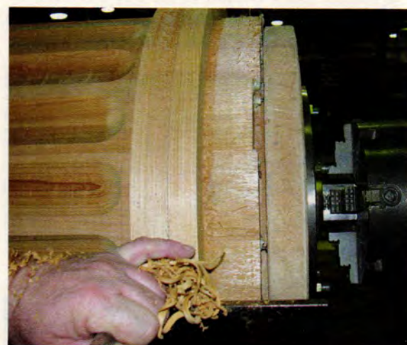
After turning and fluting, the Astragal molding of a wood column is hand turned at the top of the wood column shaft by workers at the Somerset facility. Photo: Somerset
