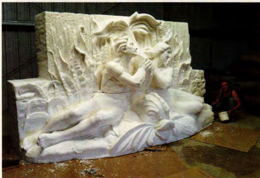
Andrian Melka is hand sculpting lost detail onto the foam model. Photo: Nathan Hunt
