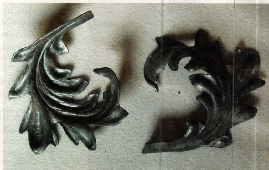
Fine Architectural Metalsmiths repoussed these finely detailed acanthus leaves to replace the original leaves on a gate.
