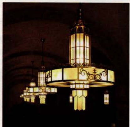
These reproduction fixtures were fabricated by Lighting Nelson & Garrett for CIBC Mellon offices in Toronto, Canada; they were re-created in solid brass and leaded glass using archival photos from an 1930s architectural magazine.
