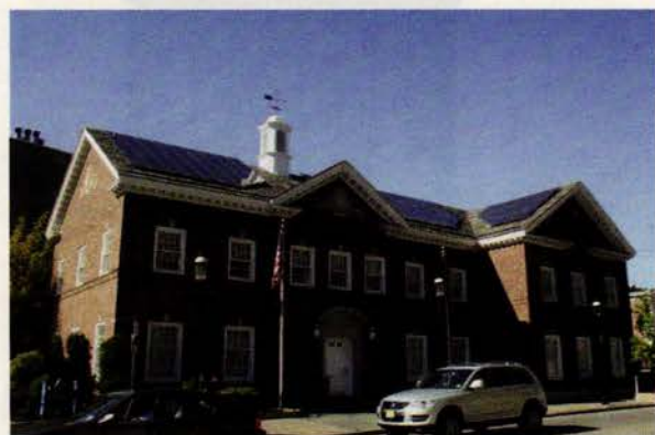
What not to do: While the goal is laudable, the prominent solar panels on this building present two potential problems: (1) They are clearly visible from the street and compromise the building's historic character, and (2) The mounting brackets for the panels could eventually cause roof leaks. Photo: courtesy of Voith & Mactavish
