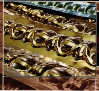
With the only two Pneumatic Gravity Drop Hammers in the New York Metropolitan area, we are able to create exact reproductions of existing designs that are identical to the **ORIGINAL** and meet strict landmarked specifications. Stampings can be made to replicate new designs or from drawings and photographs of original pieces that no longer exist.
