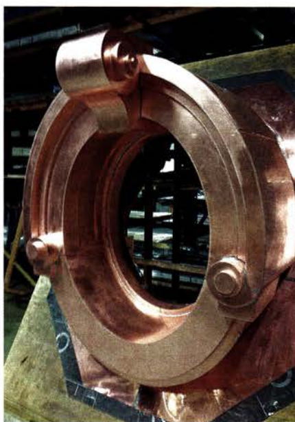
Gotham Metalworks created this copper-covered oriel window, taking into account the complex angular geometry and the integrity of the building's original architecture. Click on no. 2042
