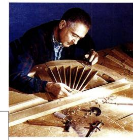
This artisan from Timberlane is putting together a solid kiln-dried western red cedar shutter using mortise-and-tenon joinery.
