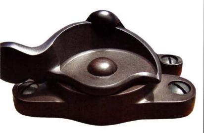
The model LKF18 sash lock from Phelps Company is hot-forged from solid brass and CNC machined; it features a double stainless-steel spring mechanism for smooth operation.
