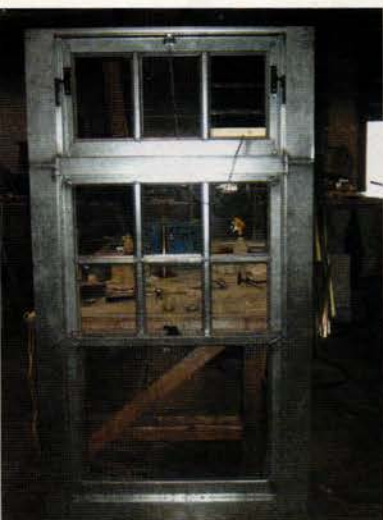
This hollow metal window was built by Heather & Little for the Roebbling Museum in New Jersey.
