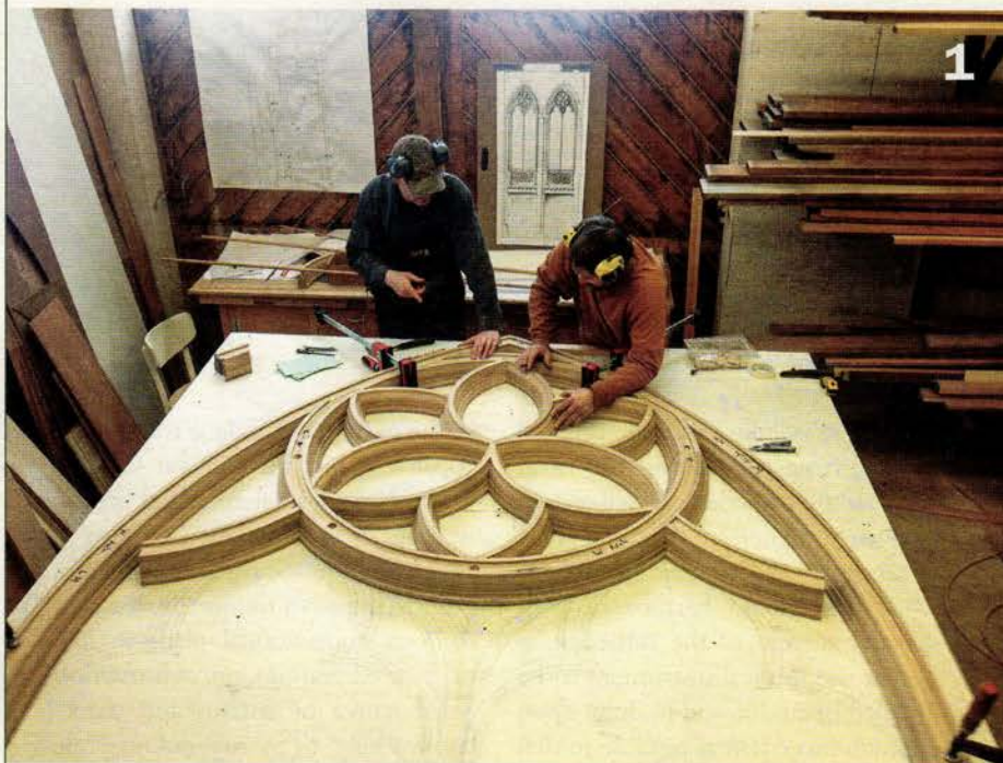
1: The main arch tracery underway in the shop. Note the scale of the woodworking compared to the craftsmen, and how the circular rose will be supported by the lancet arches to come.
