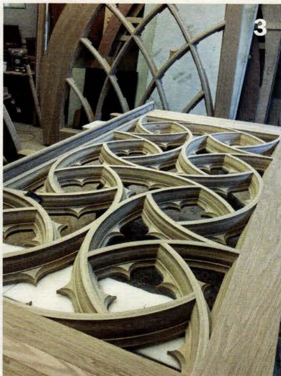
1: The main arch tracery underway in the shop. Note the scale of the woodworking compared to the craftsmen, and how the circular rose will be supported by the lancet arches to come.
