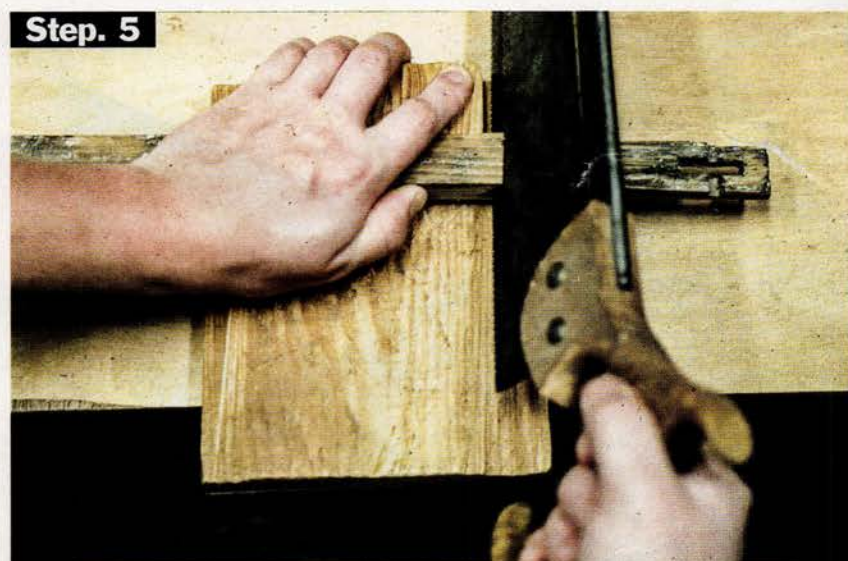
The stile socket is shaped with traditional woodworking tools.
