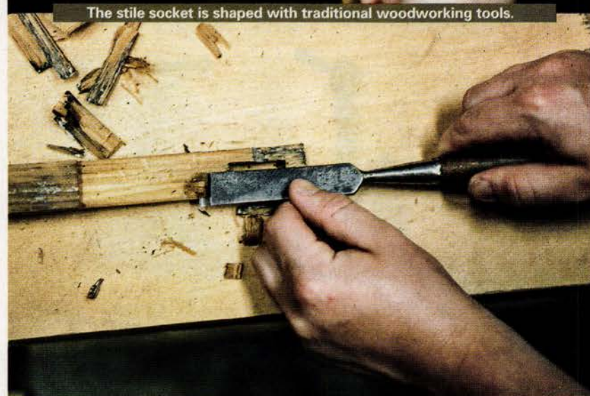
The stile socket is shaped with traditional woodworking tools.
