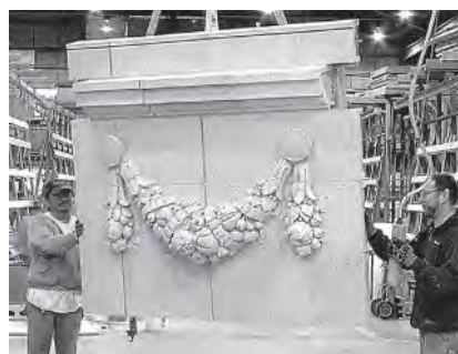
The original terra-cotta cladding on the 1916 Utah State Capitol was removed and restored or replicated by KEPCO+.
