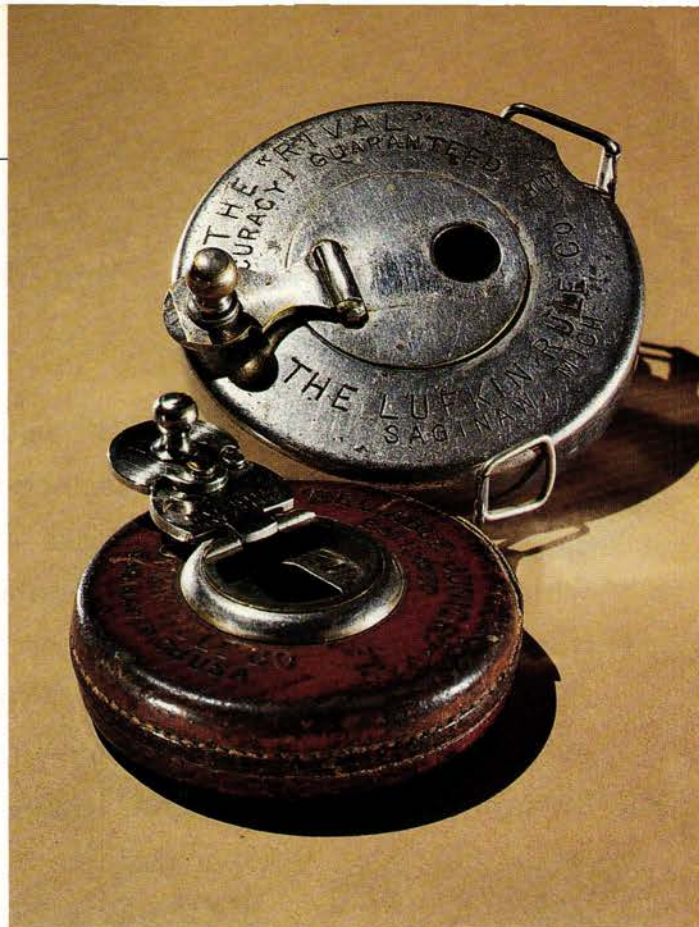
Before self-retracting steel tapes, hand-cranked models measured long distances. "Reliable Junior" of 1893 has a leather case and pop-out winding handle. "The Rival" is newer. Both measure 25 feet.
