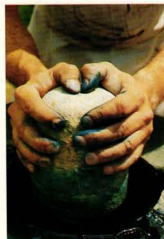
Circular action with a stone muller melds oil and pigment.
