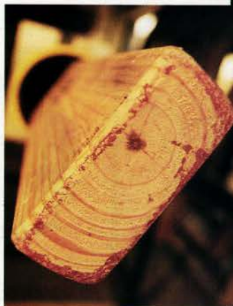
ABOVE: New windows or shutters are tested in a laboratory equipped with an air cannon. LEFT: The cannon shoots a 9-pound 2x4 at 34 mph. Windows or shutters also must withstand winds of at least 110 mph through 9,000 gusts. Glass is allowed to break under this abuse, but it must hold together and remain in its frame.
