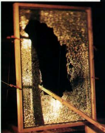
ABOVE: Laminated glass, made with a polyvinyl butyral layer in the middle, passes the 2x4 test. This glass is similar to that used in automobile windshields.
