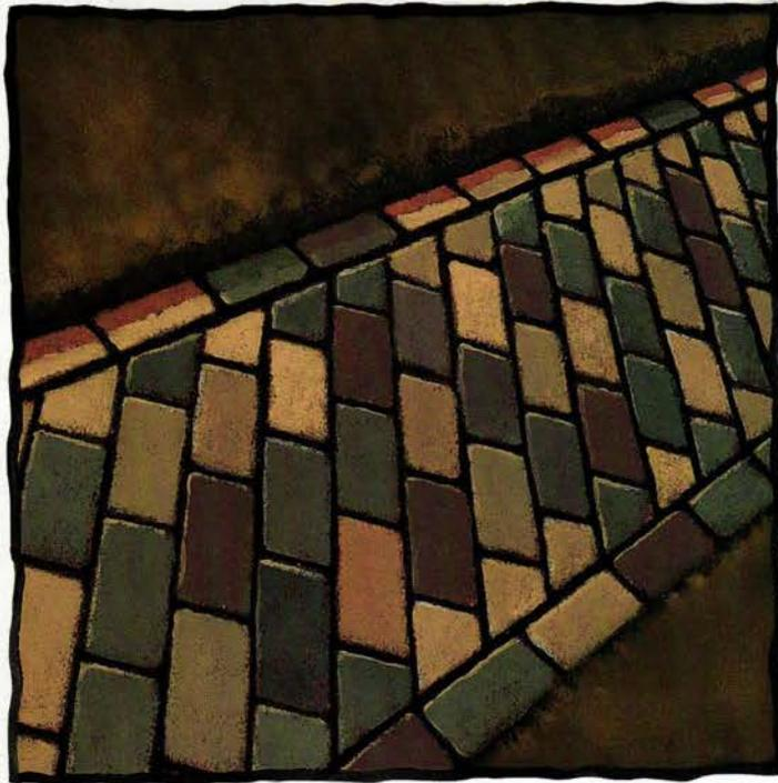
A traditional pattern twisted to the diagonal is edged with bricks laid flat, called a stretcher course in masonry work. The design requires a significant amount of custom cutting.
