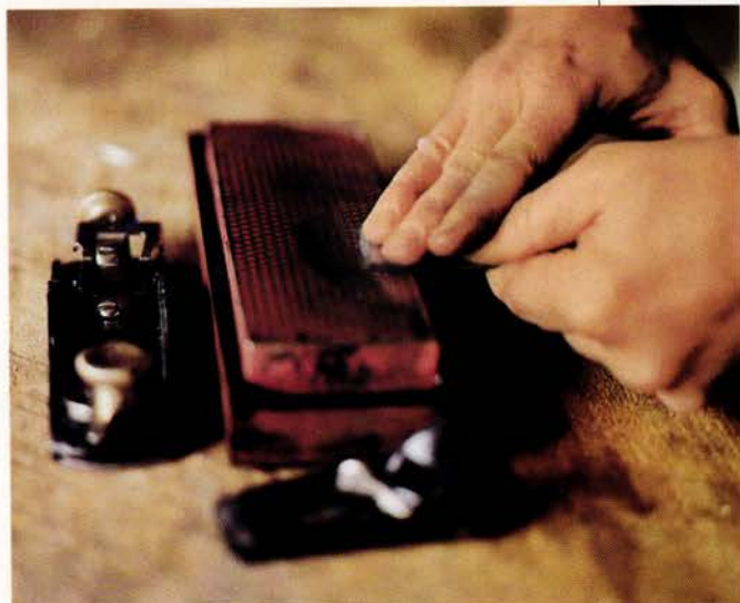
Before Norm sharpened this new iron, the back was rippled with tooling marks from the factory. But after a few minutes on his diamond stone, a mirror finish shines instead.
