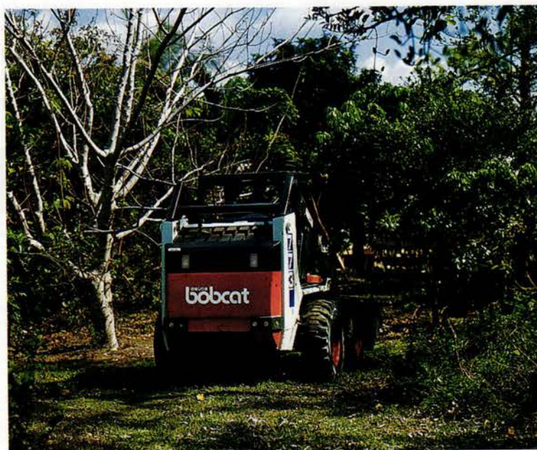
Hydraulic drives on each side allow these earth-movers to thread nimbly among obstacles that might stymie bigger machines.
