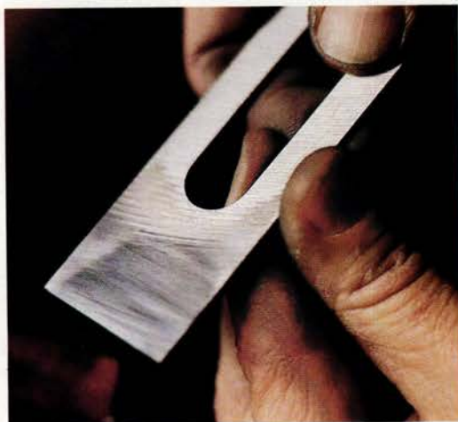
Before Norm sharpened this new iron, the back was rippled with tooling marks from the factory. But after a few minutes on his diamond stone, a mirror finish shines instead.
