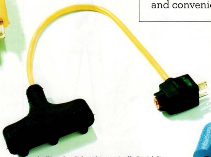
In-line circuit breakers cut off electricity when the load exceeds a preset amperage. Once the overload is remedied, power can be restored with the push of a button. Unlike GFCIs, these are designed to protect wiring, not humans.
