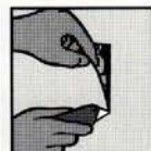
6. Trim mat at outlets, switches, etc.
