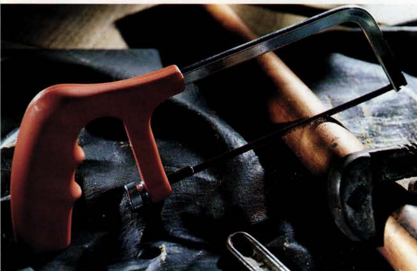
Not just a toy for craft projects, a 6-inch pony saw can hack the fine work when a full-size model would be too much tool. This model uses scrollsaw blades with pins.
