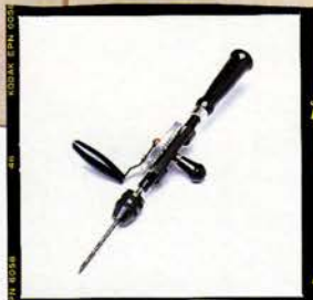
Hand drill: The egg-beater design works with small-diameter bits. For larger holes, use a brace.
