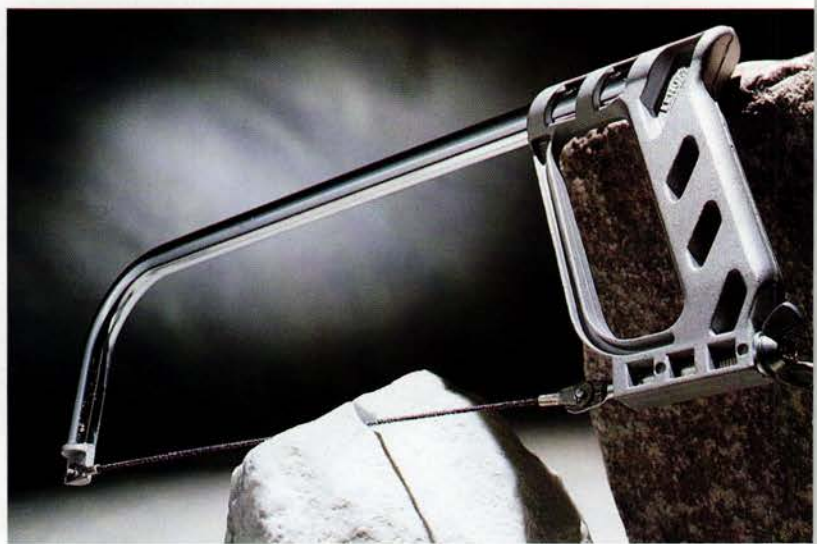
This saw combines modern features like a chromed-steel tube frame and a textured cast-aluminum handle with yesterday's blade-tensioning: the old-fashioned wing nut.
