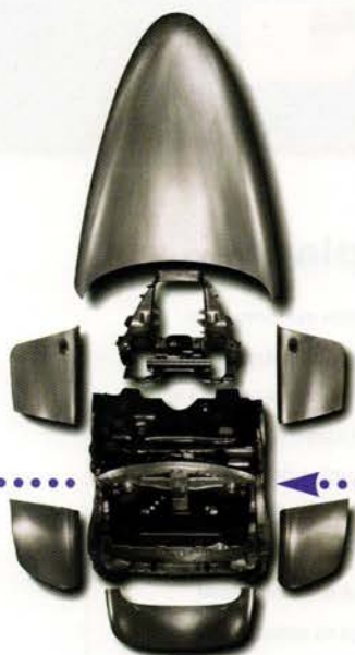
April 15, 1995: First prototype body parts, fabricated entirely from aluminum, are delivered.
