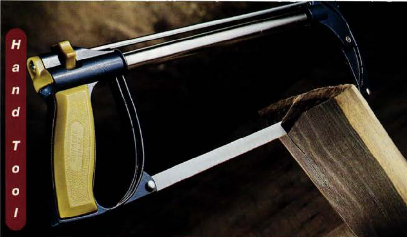
A top-mounted tensioning system combines a thumbwheel, threaded rod and an articulated lever arm to make adjustments easy. Change blades carefully: When tension is released, the pins holding the blade often fall out.
