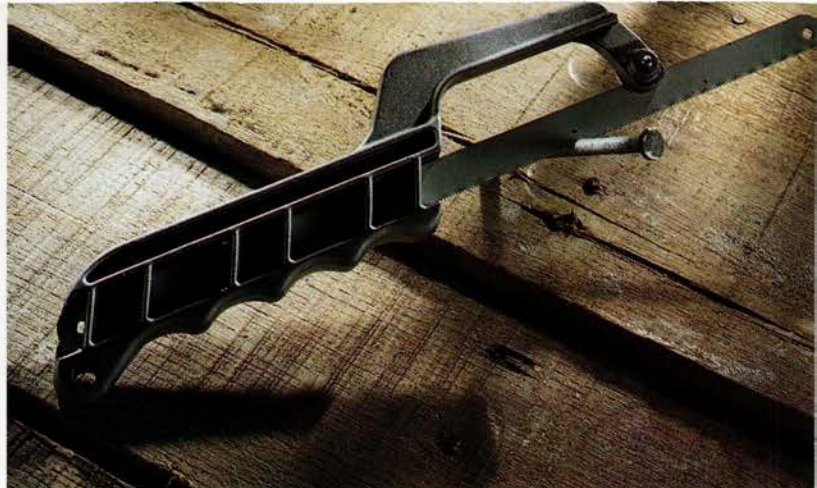
Mini or frameless hacksaws work well in tight quarters. Mount blades to cut on the pull stroke to compensate for their lack of stiffness. These frames extend the life of other hacksaws' retired blades, which are seldom worn down on the ends.
