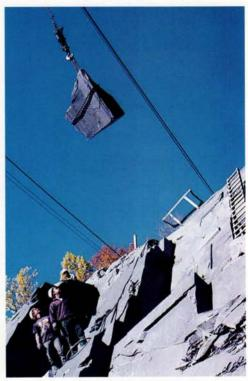
A chunk of raw slate rides to the quarry lip on a 2-inch-thick steel hoist cable towed by a turn-of-the-century crane. The crane operator can't see into the pit; he depends on signals from a bell ringer in the quarry.
