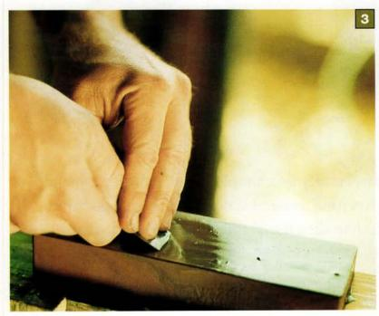
Grinding leaves a sharp but weak-edged blade, so the final step is to create a second sharpening bevel. Sharpening should be repeated whenever the blade is dull. Begin by placing the bevel's face on a medium stone set on
