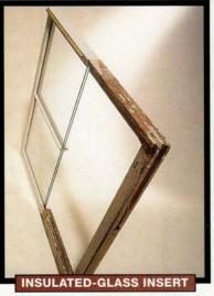
Fits into the existing sash after a bigger groove is cut in the wood. If multipane windows have muntins too thin for this groove, imitation spacers can be fitted in.
