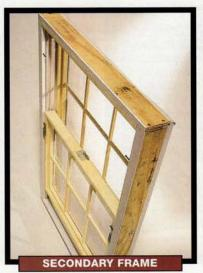
With a new sash, fits into the space where the old sash used to be, so glass size is smaller. Appropriate when the existing frame is sound but not necessarily square.
