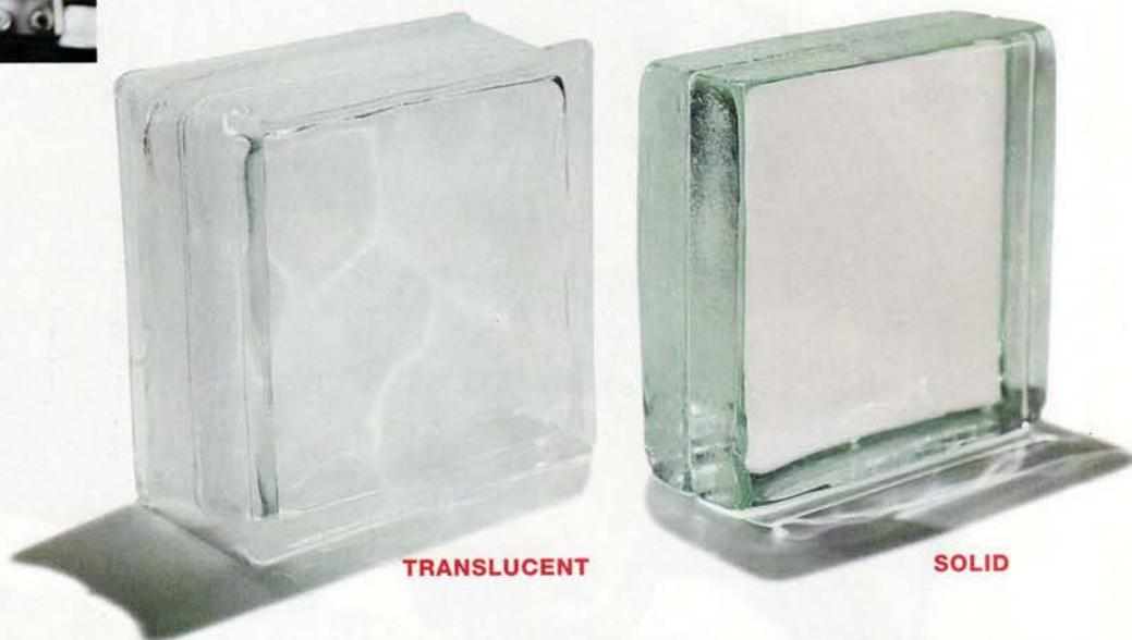
All glass block is not created equal. The LX block at left has a fiberglass scrim sealed across its center to improve energy performance, minimize heat gain and muffle noise. The Vista Brick, right, a solid 3-inch-thick chunk of glass weighing 15 pounds, is made for demanding situations. It will withstand a 1,500-degree fire for 90 minutes and stop a .357 magnum bullet. Plus, it is 32 percent better at reducing noise than its hollow cousins.
