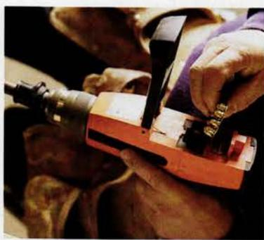
When it's time to reload, Tom opens the cover and drops a 10-load wheel into the gun. Pins are inserted one at a time.
