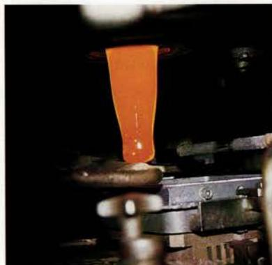
ingredients are heated to 2,600 degrees Fahrenheit in a brick-lined tank. Then a teardrop or “gob” of molten glass, above, is cut off and dropped into an open cast-iron
