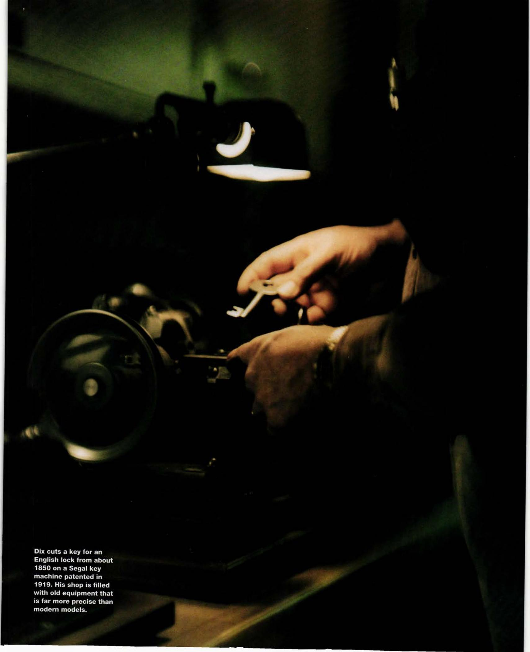
Dix cuts a key for an English lock from about 1850 on a Segal key machine patented in 1919. His shop is filled with old equipment that is far more precise than modern models.
