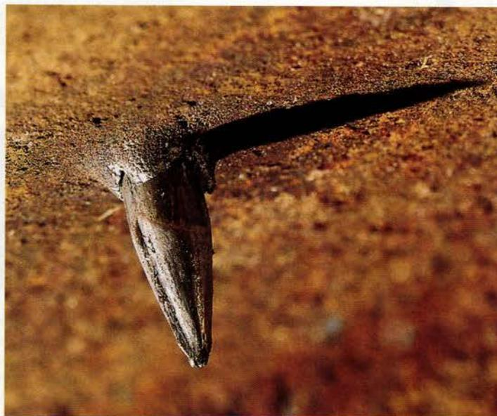
**A pin shot perfectly into steel penetrates just past the taper. The steel grips the pin shaft in a tenacious, nearly unbreakable hold.**
