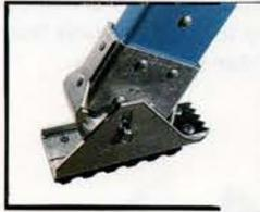
An extension ladder should always be set against a wall with the moving half—the fly section—on your side. A rope and pulley haul it up and flippers lock it in place. This industrial-grade ladder has fiberglass rails and steel shoes with picks that jam into soft ground. Fiberglass is strong and safer around wires than aluminum, but it's heavier. Sunlight degrades it, exposing fibers and letting in moisture. If the surface is damaged, spot-cover with polyurethane paint.
