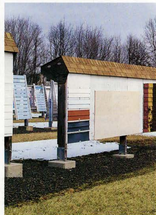
At the Paint Quality Institute near Philadelphia, odd-looking fences test how paint performs on wood, aluminum and even faded vinyl siding.
