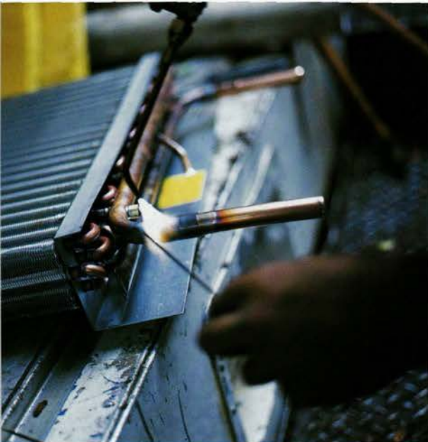
The heat exchanger looks like a car radiator and works like one too. It takes heat from the Triathlon's engine and puts it into the house's air ducts, sometimes providing more than half the unit's heat output.
