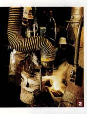
brass—an alloy of copper, tin and zinc heated to 2,268 degrees. 3. Minutes later, when the brass cools enough to hold its shape, the mold is shaken loose and Jorge Tellez grinds and polishes the still-hot casting
