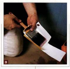
Wrap bristles in a keeper so they stay straight. Store flat or hang. Brushes for some latex paints also need a dip in a water-rinsing solvent after a soap-andwater wash to rid the filaments of residue.
