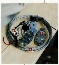
Using the cable kit provided, Tom Silva threaded the stainless wire (1) through metal eyes (2) on the bay's ceiling and seat and bolted one end to the seat bottom. He laced the other end through a zigzag tie-down (3) and easily pulled it tight. Interior trim nailed over the mullions hides the cables, disguising the fact that anything is holding the bay aloft.
