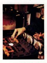
black sand. Atop each gritty depression, he places a delicate core of finegrained white silica, which will form the faucet's hollow waterways. 2. After Castro mates the two halves of the
