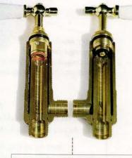
From the outside, both valves look the same, but the left one turns a ceramic disc, while the one on the right compresses a rubber washer against a metal seat. Super-smooth white ceramic discs, below, made of aluminum oxide, promise long, leak-free service; old-fashioned washers are cheaper and easier to replace.
