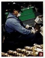
plating, which covers the casting with a nickel coating onethousandth of an inch thick and a chrome topcoat one-millionth of an inch thick. The plated spout is then married to valves machined from
