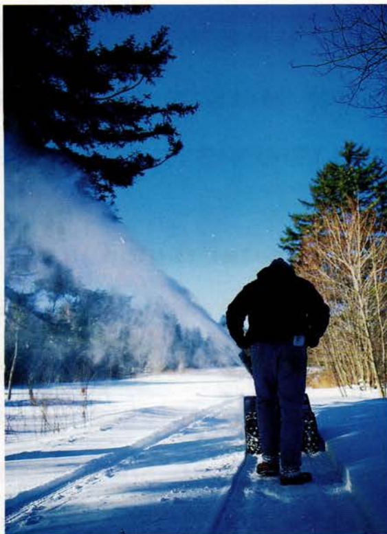
A few inches off the top: When the mailbox is 900 ft. away, you don't need a major blizzard to justify a snow thrower. The track-drive Honda, shown throwing a rooster tail of fresh Vermont powder, offers three ground-clearance settings that let you choose how close a shave you want.
