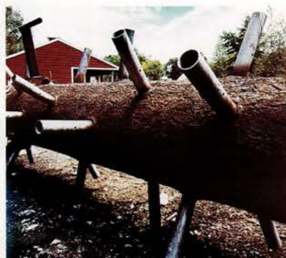
Epoxy resin molded like bark coats a steel shaft, and plastic branches fasten on.
