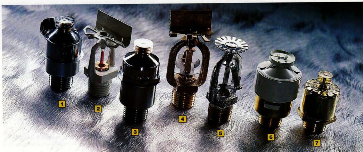
Some residential fire sprinklers (A) are concealed behind caps that pop off during fire; others (B) hang exposed. The big risk with covered sprinklers is that someone will paint over them, filling the tiny air space between cap and ceiling that devices need to trigger promptly. Bare sprinklers have their own downside—they’re too handy for coat hangers and mobiles. Some sprinklers (1, 2 and 4) can be installed on walls, 4-6 in. below the ceiling. The other sprinklers are ceiling pendants in a variety of finishes.
