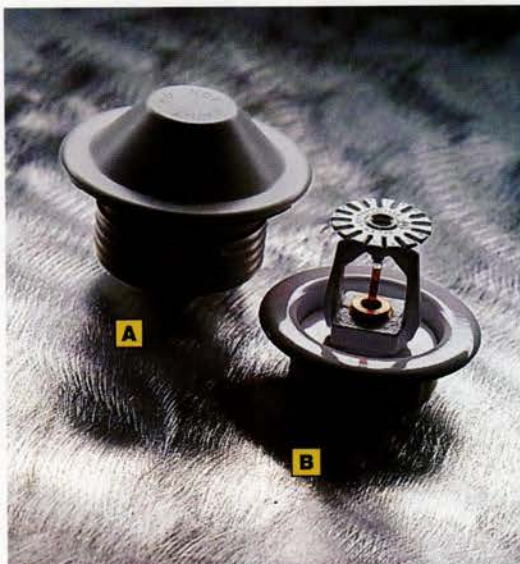
Some residential fire sprinklers (A) are concealed behind caps that pop off during fire; others (B) hang exposed. The big risk with covered sprinklers is that someone will paint over them, filling the tiny air space between cap and ceiling that devices need to trigger promptly. Bare sprinklers have their own downside—they’re too handy for coat hangers and mobiles. Some sprinklers (1, 2 and 4) can be installed on walls, 4-6 in. below the ceiling. The other sprinklers are ceiling pendants in a variety of finishes.
