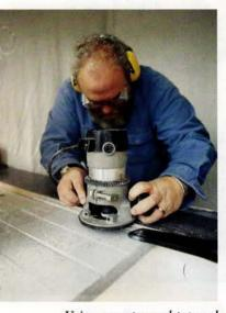
Using a router and tapered jig, Glenn Bowman, owner of Vermont Soapstone, carefully carves drainboard grooves into the soapstone counter.
