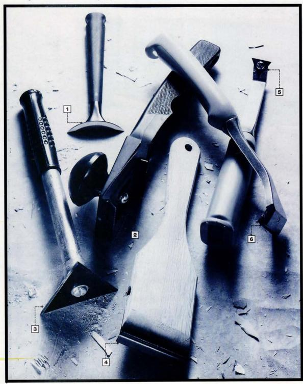
go into the corners of tiny little reveals or scrape down bowling alleys with equal ease, and the blade can be switched to its sharper edge when it gets dull. Most modern pull scrapers have removable blades with two or more edges, in widths from 1 to 5 inches.
