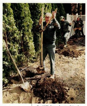
David Gladstone shuns traditional posthole diggers, which look like giant hinged chopsticks. His Gibbs Digger has a blade that swivels from vertical to horizontal with the flip of a short lever. Constant digging and sharpening wear the blade to a nub every nine months.
