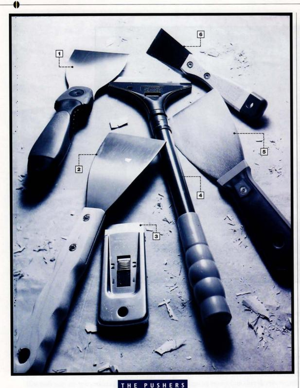
On painted wood, push scrapers work best with a heat gun or chemical stripper. If pressed too
