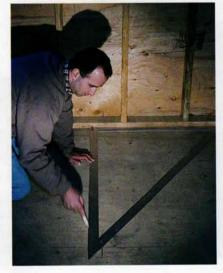
Butwin tinkered in his workshop and came up with a lightweight alternative: an anodized aluminum version that slides open and locks into place. When the job's done, the triangle folds in on itself to resemble a single narrow cross-country ski, making it a lot easier to store than a big T square.
