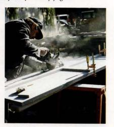
Unlike other types of stone, soapstone can be cut with an ordinary circular saw that is fitted with a masonry blade.
