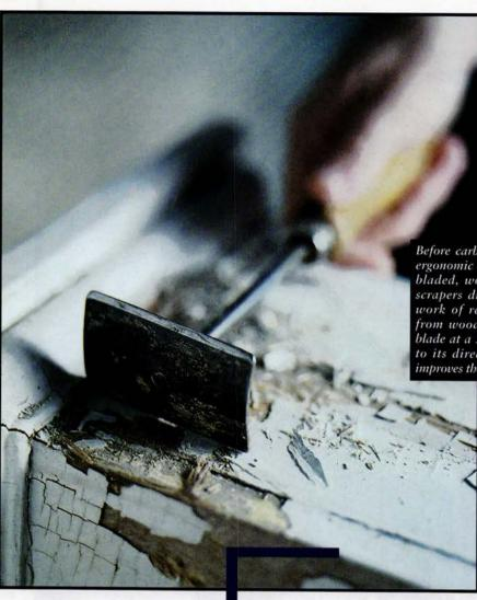
Before carbide blades and ergonomic bandles, thickbladed, wooden-bandled scrapers did the donkeywork of removing paint from wood. Slanting the blade at a 30-degree angle to its direction of travel improves the peeling action.
