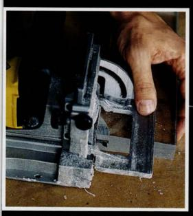
A biscuit joiner's carbide-tipped blade plungecuts a balf-oval slot into synthetics such as solid-surface countertops or Lucite, above, but the tool is most often used to bold wood together.
