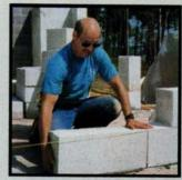
aerated concrete blocks by Hebel (photo, above) weigh 20 percent less than standard concrete, so they cost less to transport and are much easier to move.
