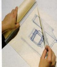
nail gets hammered, architects go through reams of the stuff, drawing scads of ideas. As they try out positions of closets, windows, French doors and so on, they can stack the drawings on top of each other two or three at a time to visualize every possible configuration. For best results, use a light touch and a marker or soft pencil to keep from ripping through a scheme taking shape. Furious activity is no substitute for understanding. –H.H. Williams
