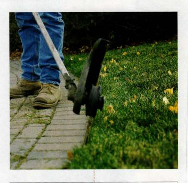
Cook trims encroaching grass near walkways by tipping his string trimmer up on edge. The tricky cut takes practice, however, because the string kicks up dirt if it dips too low. This kind of trimming calls for a firm grip and a steady gait with elbows held close to the body so that only the tip of the line touches the grass.
