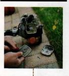
Clogged air filters choke engines dead. After four hours of trimming, rinse in soapy water and dry.
