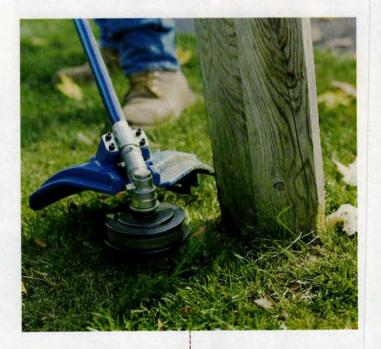
When trimming near woodwork, always know where the tip of the string is—or your post will be toast. The flailing string can wear through finishes, peel wood shards or leave unsightly rings of wear. Trimming too close to rock also wears out the string prematurely. The string should kiss the obstruction, not whack against it.
