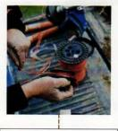
When rewinding heads, keep coils snug and parallel to prevent string from fusing to itself.
