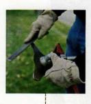
Brush blade too dull? Sharpen cutting edges with a flat file. If the blade is bent, replace it.
