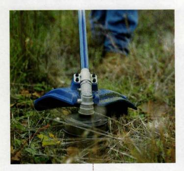
Nylon line beats a blade in light brush or tall grass, particularly if conditions are wet, because the line rarely binds up with severed strands. Cook keeps the head level and sweeps it back and forth in narrow arcs as he walks slowly forward. Swinging the trimmer too far left and right is a common mistake causing a loss of balance.
