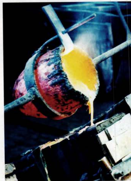
Suspended in a pouring tool operated by two foundrymen, a red-hot crucible is tipped over frames containing sand-cast doorknob molds. Molten brass rushes out, with a white-hot flame licking at the crucible's lip. "You can't stutter or stop, or the mold is ruined," says Martin Grubman, assistant to P.E. Guerin's president.
