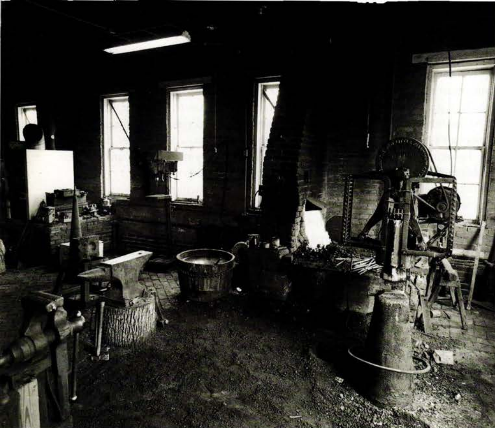
Tools and fixtures in Keller's shop include, from left, a vise, an English-pattern anvil atop a stump with hammers leaning on it, a slack tub, a brick forge, the fire, various tongs and a trip-hammer. The dirt floor traditionally accommodated horses brought in to be shod.
