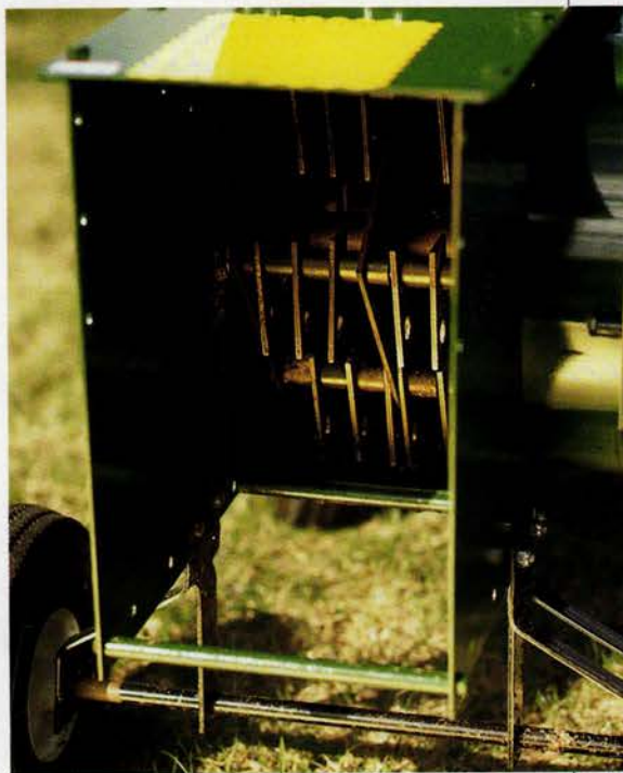
The big Mighty Mac's shredder, pictured with its protective panel removed, attacks yard and garden debris with 24 swinging hammer flails. Suspended from four rotating bars, the hammers rapidly turn branches up to 3½ inches in diameter into finely ground mulch.
