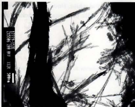
Asbestos has a fibrous structure—magnified here 12,000 times—which makes the material dangerously invasive.
