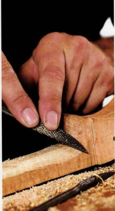
clog, because the chips slide through the tiny openings. Planing rasps were first made with tempered high-carbon steel sheets tensioned onto light cast-metal handles, top (on top of stack). Stainless steel planing rasps can be attached to a hacksaw frame or bent into shapes such as the round one furniture-maker Perry Balog uses to smooth the joint of a chair arm, bottom.
