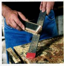
A file card has spring steel wires on one side to floss out the chunks caught in the rasp's teeth; the other side has soft nylon bristles to brush away loose dust.
