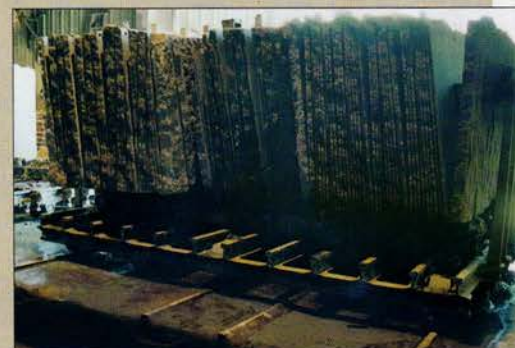
After 48 hours in the swing saw, a 25-ton chunk of carnelian granite looks like a big loaf of sliced bread. Next stop for these slabs: the polisher.
