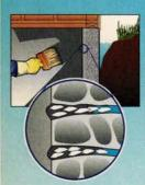
When applied on wet or damp concrete, the active ingredients in Hi-Dry penetrate deep into the pores, producing a crystalline formation which seals the structure against water seepage.
