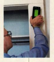
With a burst of cadmium-109 X rays, Donald Pesce's \$14,000 XRF causes any lead in the paint to emit its own signature X rays, which the device then detects.
