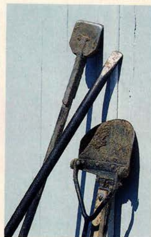
ABOVE: It takes two to set and plumb a post: While Sludock tamps the soil and keeps an eye on the level, Danny King shovels on more dirt. RIGHT: The key tools of this trade include, from left to right, a tamper, a digging rod, and a Seymour digger.
