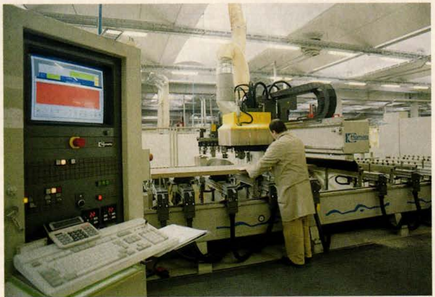
At a factory in Brianza, Italy, a modern-day cadrega (chair maker) uses computerized equipment to produce sheets of cherrywood-veneered fiberboard.
